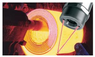
Optris High Performance sensors including the CSlaser, CTlaser and CTratio products take performance to the next level. They incorporate a dual laser aiming system enabling precise aiming of the measuring spot. The two lasers also pinpoint the size of the spot on the object being measured. Very high grade optics allow for the smallest of measuring spots. The CSvideo and CTvideo models provide simultaneous video alignment and double laser sighting for when viewing conditions are poor.
