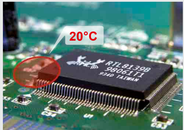
Spot size chosen too big which results in a measurement error
