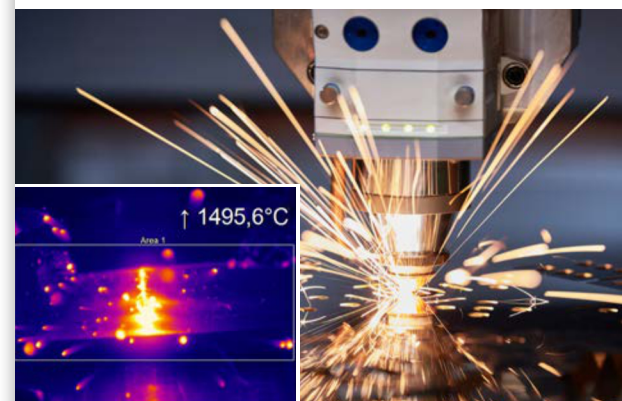
The installed PI 1M monitors the process for quality assurance
